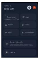
To access the Quick Settings menu, enter the Home screen by pressing the (home) button on the remote control, then press the (quick settings) button.
