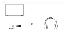
When wired headphones are connected to the 3.5mm jack socket of the TV, the internal speakers will cut out. The volume of the sound which comes from the headphones is controlled via the remote control using the [VOL-] and [VOL-] buttons.
