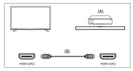
(A) AV receiver or sound bar (B) HDMI cable (not supplied)\*
