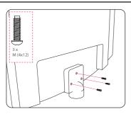
1 Attach the stand neck to the rear of the TV set using the 3 x M(4x12)
