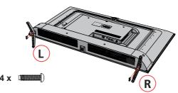
When the stand/feet are in the correct position, secure the feet to the underside of the TV set using 4 screws provided.
